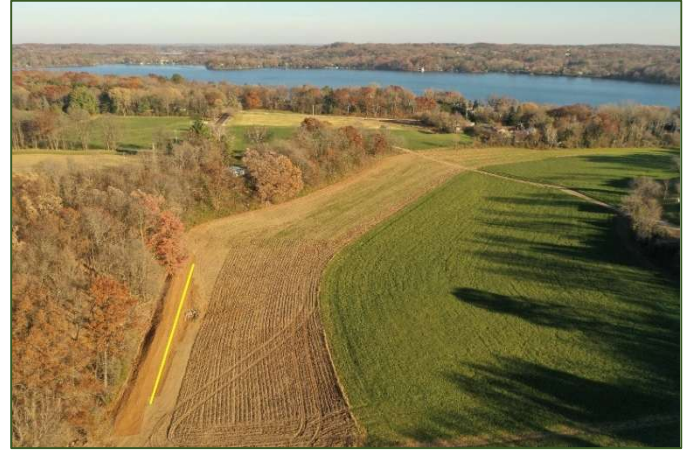
Middle field constructed WASCOB (yellow line) along the tree line. Photo courtesy of Washington County
